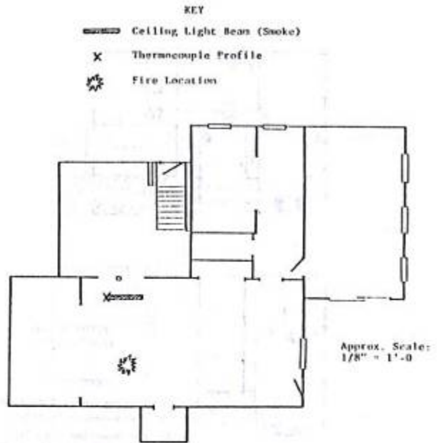
Figure 19. Fire locations and portable ignition room instrumentation on basement floor of J. R. Whitehouse residence.
